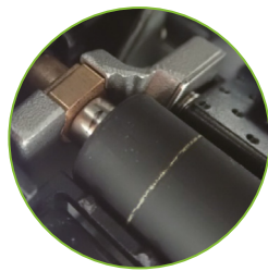
White line starts to fade when platen roller starts to wear out.
