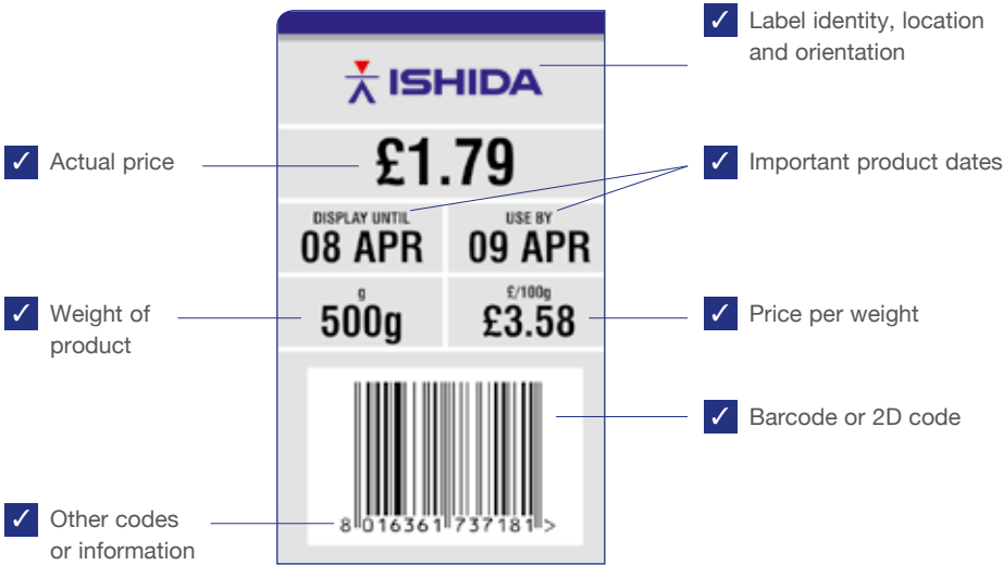
Some of the label parameters checked by the Ishida Vision System
