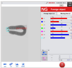
Example: Metal clips masked and counted to confirm presence. Stainless steel detected down to 0.6mm
