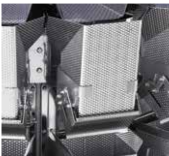
Faster opening and closing of hoppers
