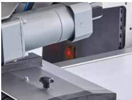
Bin full and reject confirmation sensors
