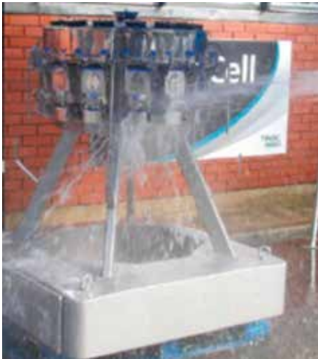
Under-going powerful water jet test for IPX6
