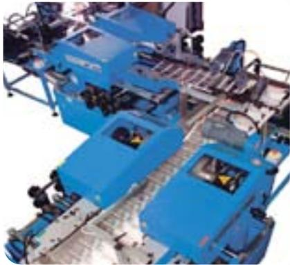
As standard, the trimmer is equipped with tempered and air cooled hard metal knives, ensuring superior trimming quality. Thanks to quick knife exchange and inexpensive re-sharpening of the knives, investment costs will be reduced.
