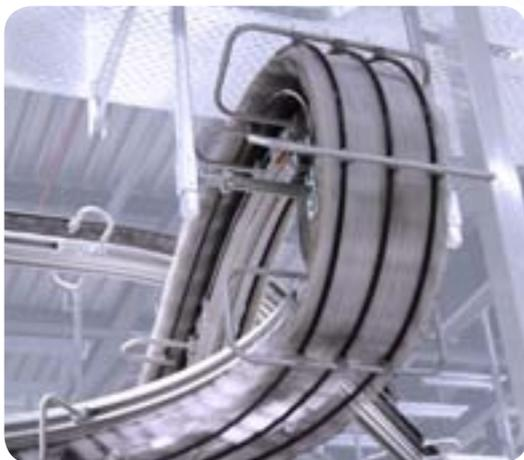
The transport and release is highly reliable and free from interruptions. The contact area between the gripper and the copy is held to a minimum and the connecting points are widely spread apart to secure ensure gentle handling and reduce the risk for smudging to a minimum.
